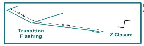
End Laps Min. 8" W/ 2 beads of concealed sealant.
