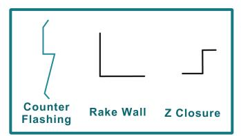
Minimum 4" Overlap with continuous concealed sealant
